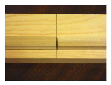
The straight, factory edges should meet in the middle of the base board. (You can measure and mark a line across the middle to help). Leave a small gap just big enough for your hack saw blade to slide inside.
