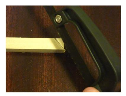
Use your hack saw to carefully cut the dowel rod straight along the 45\* angle line you just drew.
